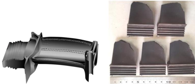
**Fig. 8** Examples of blades in a gas turbine
